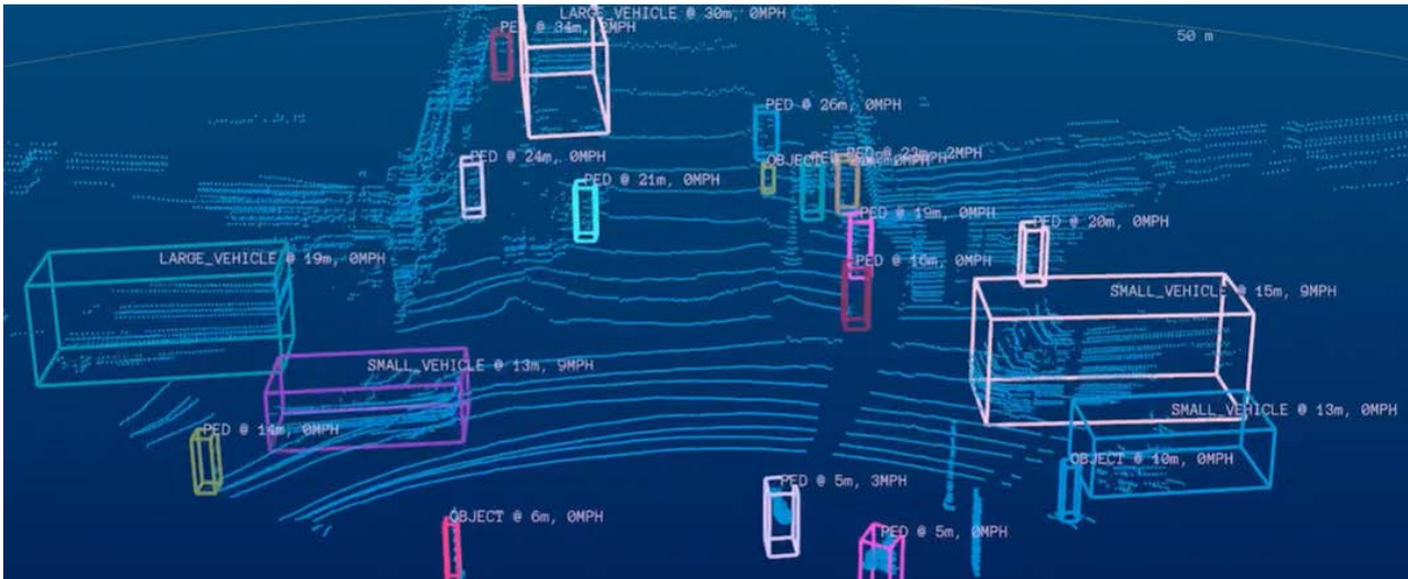
Figure 80: Snapshot from Velodyne VDK homepage, which shows classification of objects from a point cloud in real time [10].
