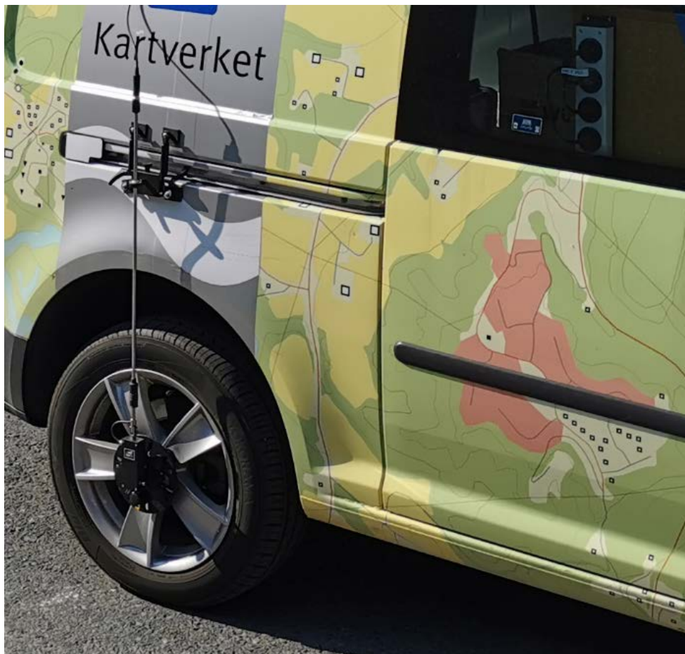
Figure 75: Pegasem WSS2, a mechanical rotary and incremental odometer, mounted on the Norwegian Mapping Authorities car.
