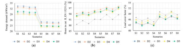
**Figure 4.** Results of the three performance indicators for the five analysed designs across the eight scenarios: (**a**) Energy demand results (including only heating, cooling, and lighting). (**b**) Thermal comfort results (average % of hours in cat. II of EN 15251 in five main rooms). (**c**) Load cover factor results.
