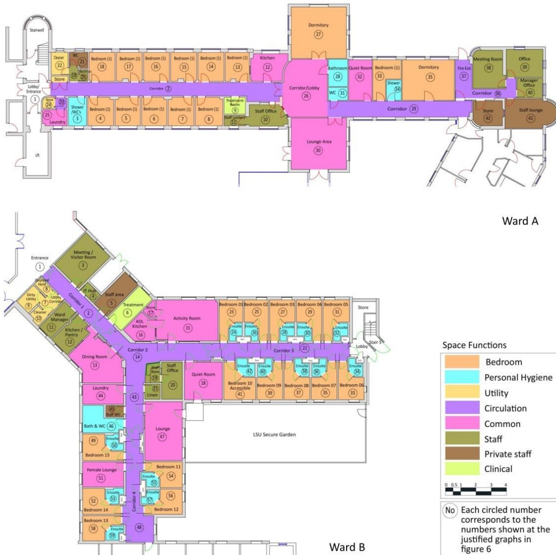
Figure 5. Floorplans of Wards A and B. The architectural drawings are color-coded according to functions
