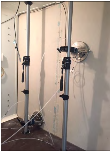
Figure 2. Installation of the FLECs on the constructed wall for VOC measurements
