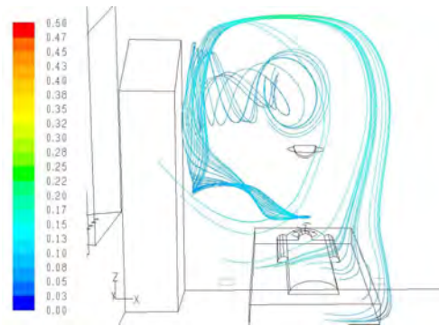
Figure 8a. The path lines of the particles in the ward colored by particle velocity magnitude (m/s) with only one patient (left) releasing particles.
