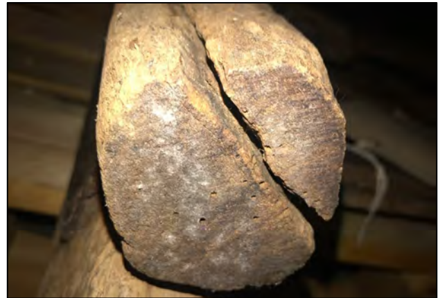
Fig 8. A wooden tool with fungal growth (repository 3)
