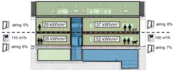
Figure 9. Total energy use in one year for heating and cooling the apartments. Also shown are the airing factors averaged over the whole year. Conditioned spaces are coloured green and unconditioned spaces are coloured blue.
