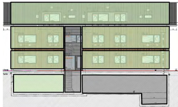
Figure 1. The building with the conditioned areas that can be heated and cooled (green) and unconditioned areas (grey).
