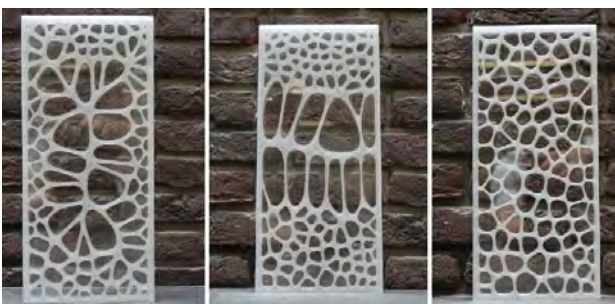
Figure 3. Glass panels (3D-printed PETG Voronoi core) (Neeskens, 2018)
