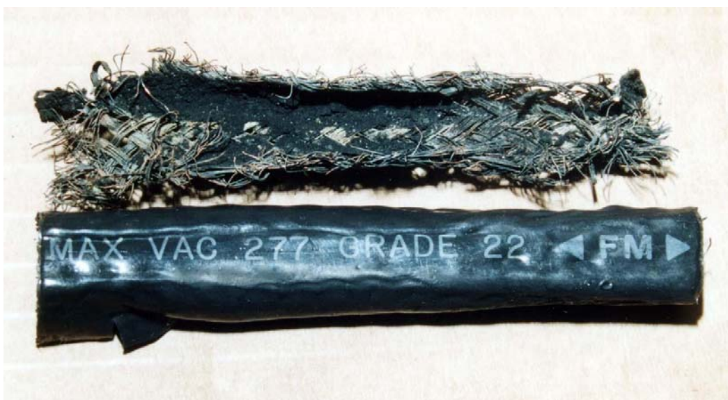
Figure 10: A piece of the cable from Heidrun. Overjacket is removed and braid opened. Both conductors are disappeared.
