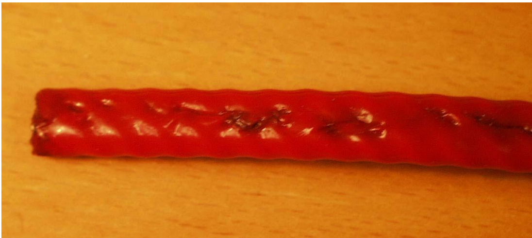
Figure 22: A piece of cable 8XTV2 with inner sheath. Distinct hotspots.
