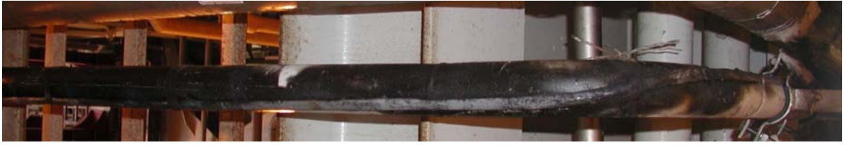
Figure 4: Same cable as shown in Figure 3. From the point of failure close to the flange the cable was burnt-out in length of four meter (from the point of failure in the direction to the coupling box).
