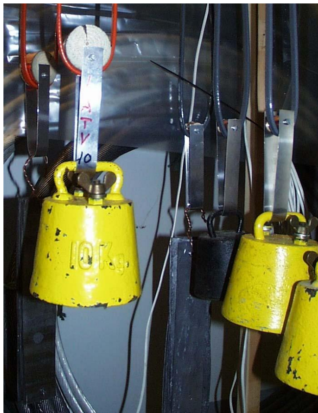
Figure 14: Tensions of 5 and 10 kg are applied to the cables by appending weights. These are hanging in circular blocks of wood with radius 12 and 28 mm.
