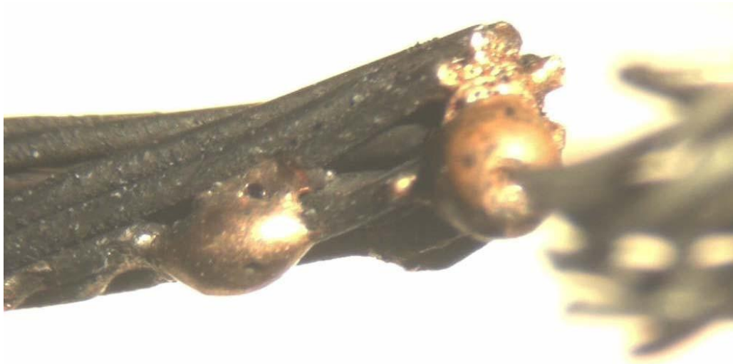
Figure 7: Microscope picture of the rupture location where a serial arc has occurred (6 x magnification).
