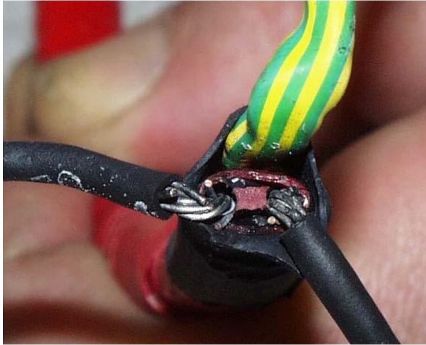
Figure 21: Cable end for voltage connection. Specified cable termination is lacking.
