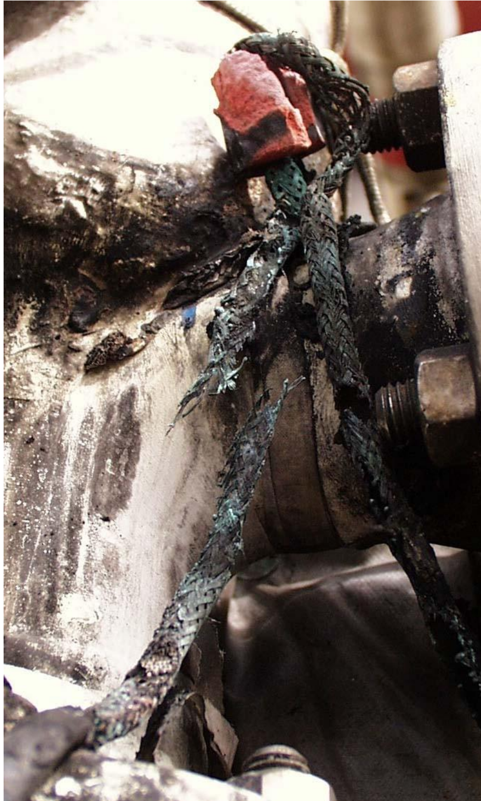
Figure 2: Same cable as shown in Figure 1. The cable is completely burnt-out, only the metal screen is left. At the same time we also see a somewhat irregular installation of the cable.
