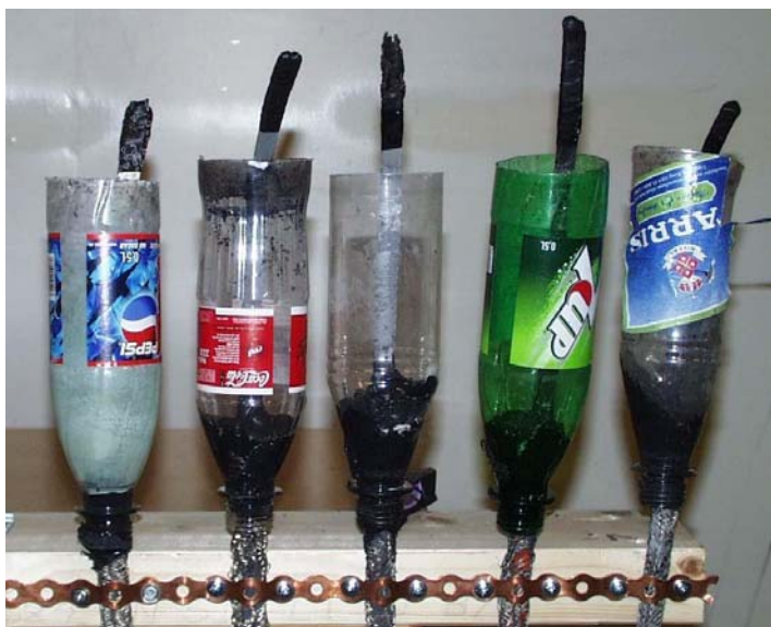
Figure 17: Examples of damaged cables. From left to right: 1: Cable caught fire in at the end. 2: Cable caught fire under the water surface. 3: Cable caught fire under the water surface and in the end. 4: Cable caught fire under the water surface. 5: Cable caught fire under the water surface.
