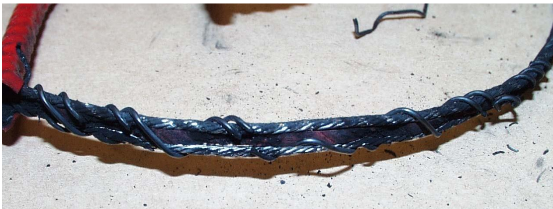
Figure 23: Cable 8XTV2 opened. There are several ruptures in the self-regulating conductive fibres “wrapped” around the live conductors. There is also plenty carbon along the whole inner part of the cable.
