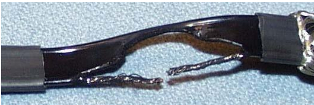
Figure 6: Combustion of the semi-conducting material in a self-regulating heating cable after a provoked serial arc.
