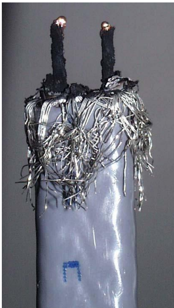
Figure 24: Cable BSX-8-2. The cutting surface was gently moistened with saline water, which resulted in glowing in the cutting surface of the self-regulating element between the live conductors. After a short time the matrix started to burn.
