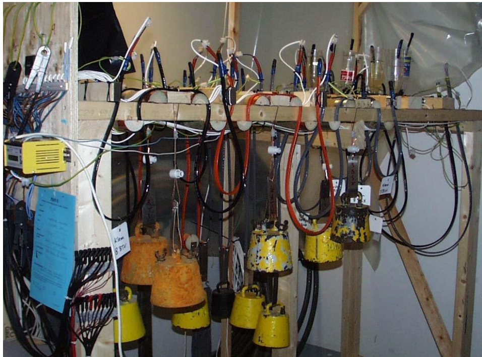
Figure 13: Overall view of cables mounted in test rig.
