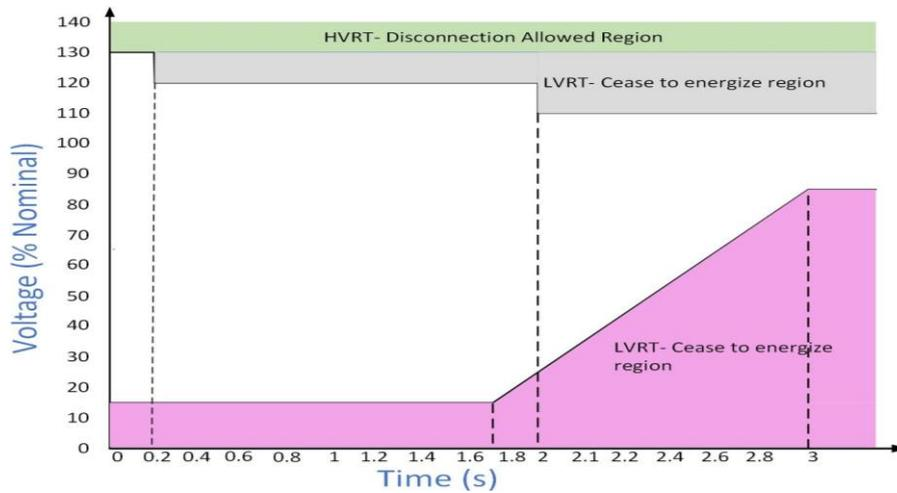
Figure 3.13 - Voltage ride through limit (X-axis values are as per CEA standard mentioned earlier). [7]
