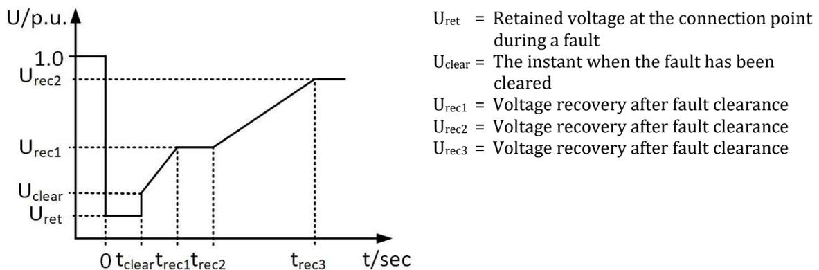
Figure 3.9 - Fault ride through curve for abnormal operation. [4]
