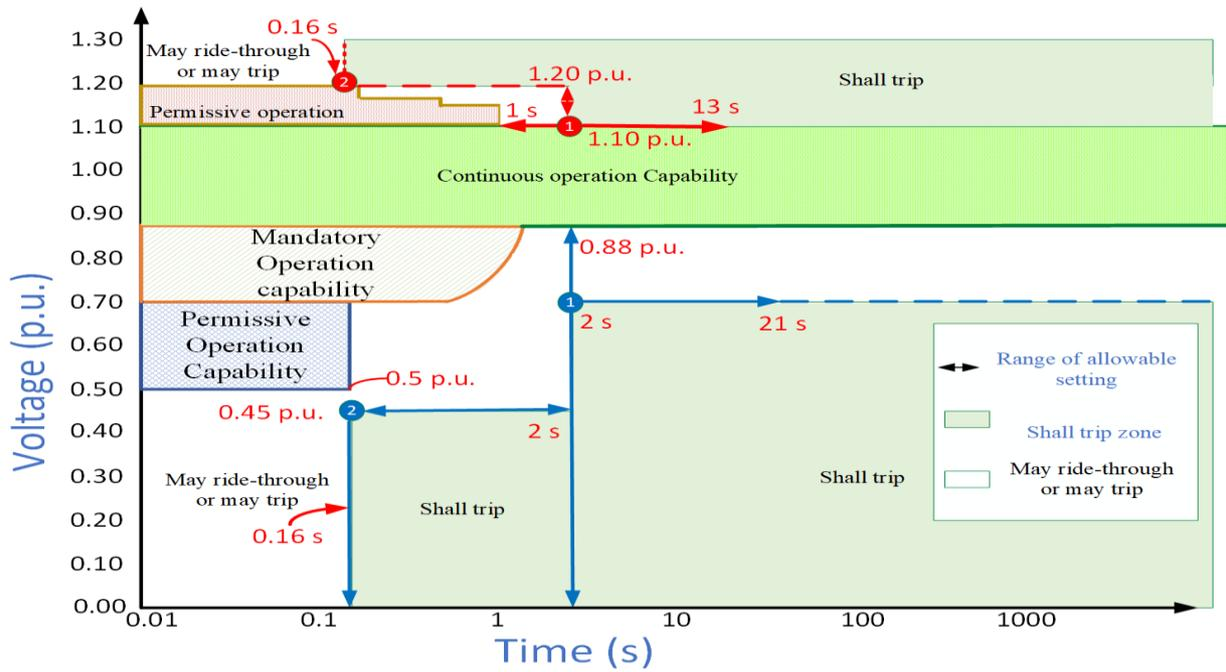
Figure 3.3 - DER response to abnormal voltages and voltage ride-through requirement for DER of abnormal operating performance Category I. [2]
