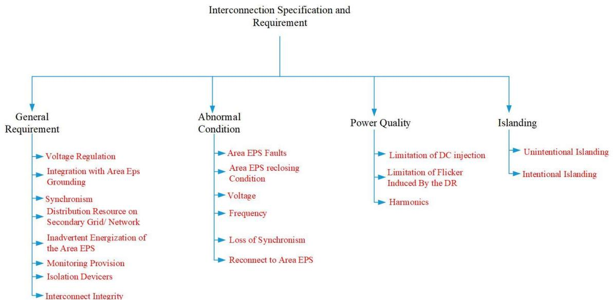
Figure 3.1 - Broad Classification of Interconnection Requirements and Specifications.
