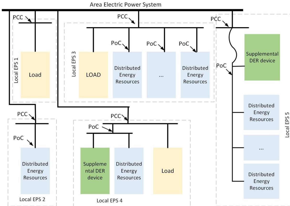
Figure 3.2 - A representative Area Electric Power System with DERs. [2] [1547-2018]
