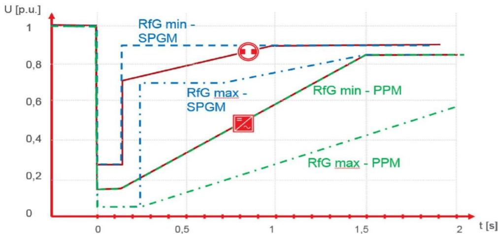
**Figure 3.11** - Voltage-time-profile for generation units of type B for synchronous (SPGM) and power park modules (PPM). Maximum and minimum limits in NC-RfG illustrated for synchronous production units (blue) and power-park units (green) Ref Statnett Reviewed RfG NC. [4]
