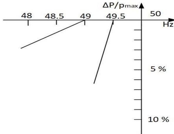
Figure 3.8 - Maximum power capability reduction with falling frequency. [4]
