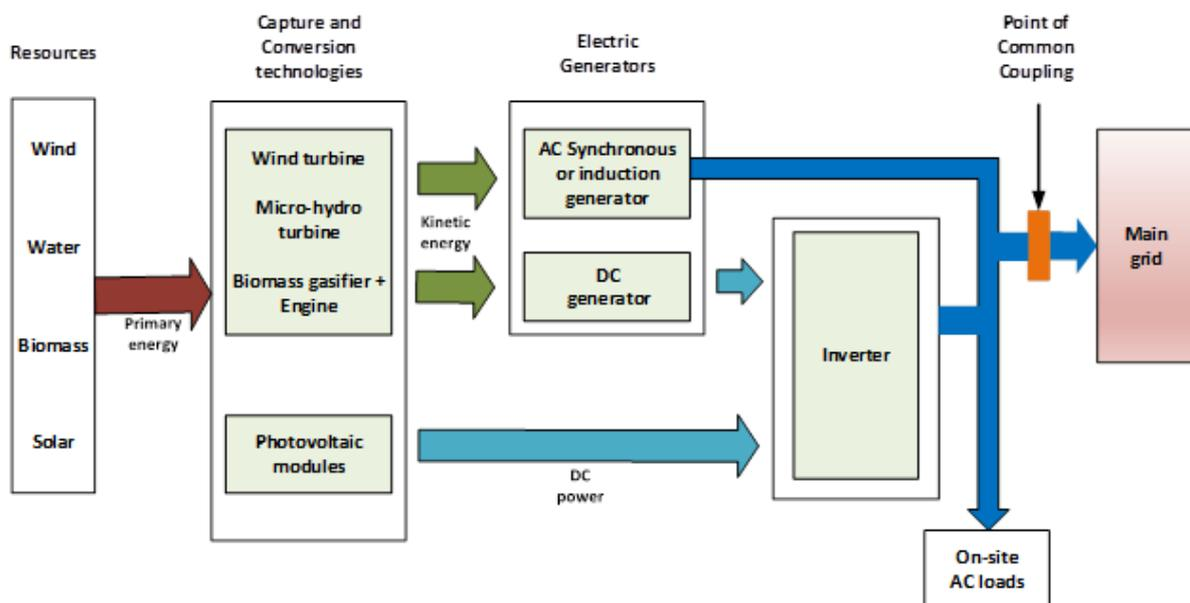
Figure 1.1 - Different types of generators connected in a renewable power minigrid [1]
