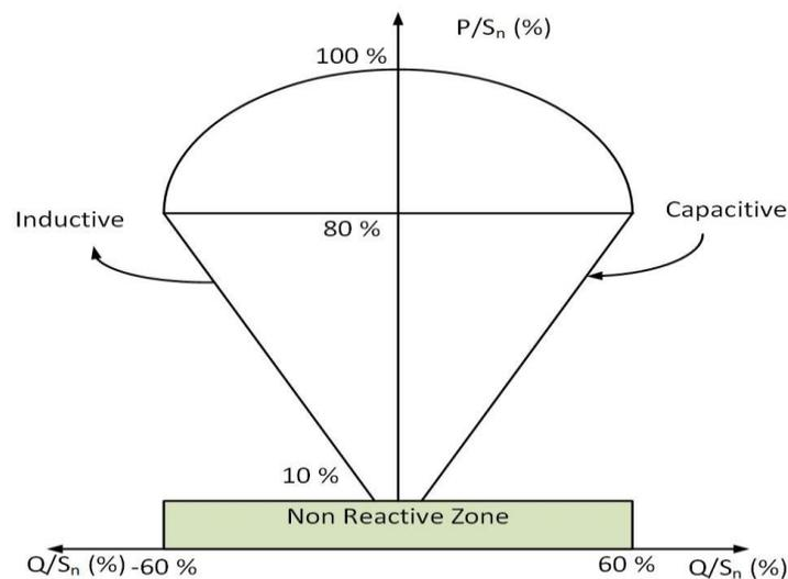
P: Active power; Q: Reactive Power;  $S_n$ : Maximum apparent Power of the inverter
