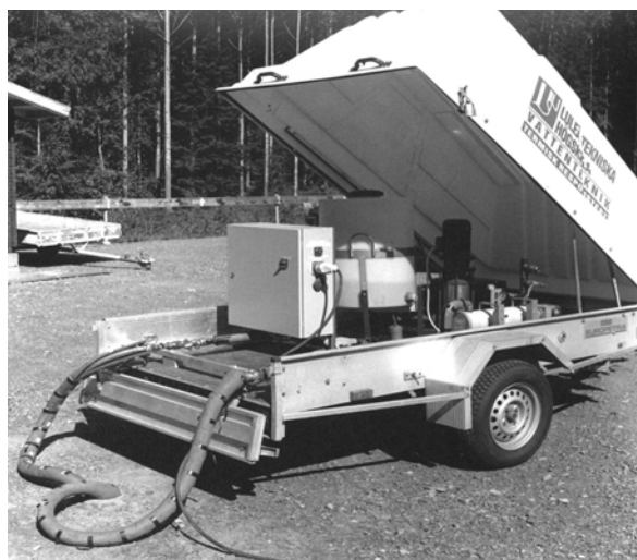
Figure 4.13 Principle of the thermal response test unit (Gehlin, 2002).
