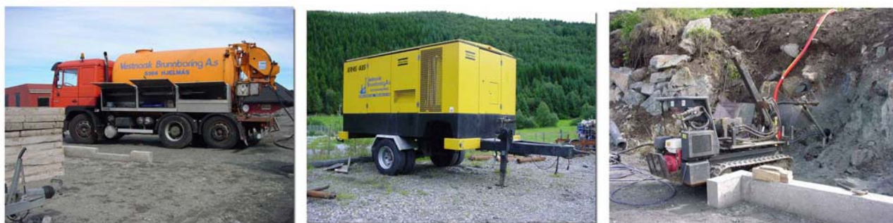
Figure 4.16 Equipment used for hydraulic fracturing of groundwater wells (Vestnorsk Brunnboring AS).
