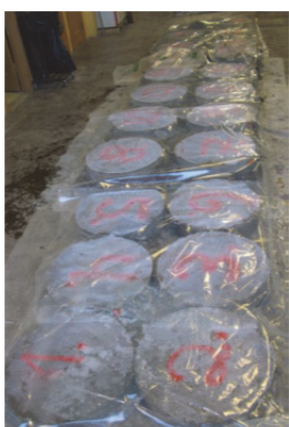
E) Numbering of panels and plastic sheet cover for curing until de-moulding
