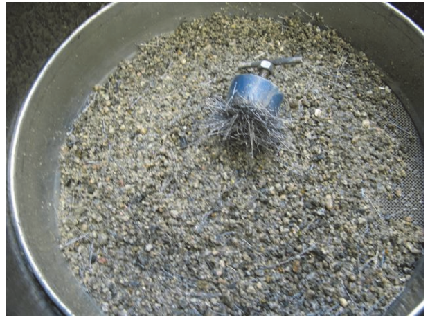
Figure 3 Fibre measurement of a 8 litre sample; 2 mm sieve, washing and steel fibre collection with magnet
