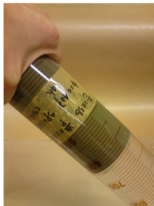
Fig. 6: “Thixotropic like” behavior of low w/p matrices (the picture was taken at 2 hours after mixing for matrix 4- wc0.56wp0.46p1.55)
