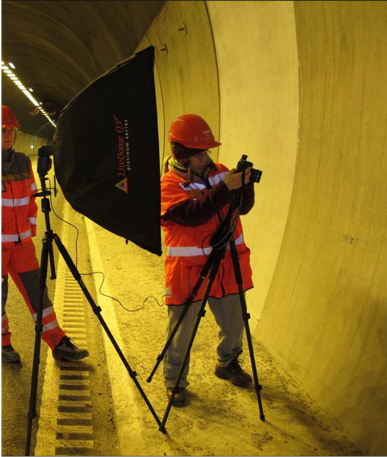
Figure 4: Set-up of camera, flash and softbox in tunnel
