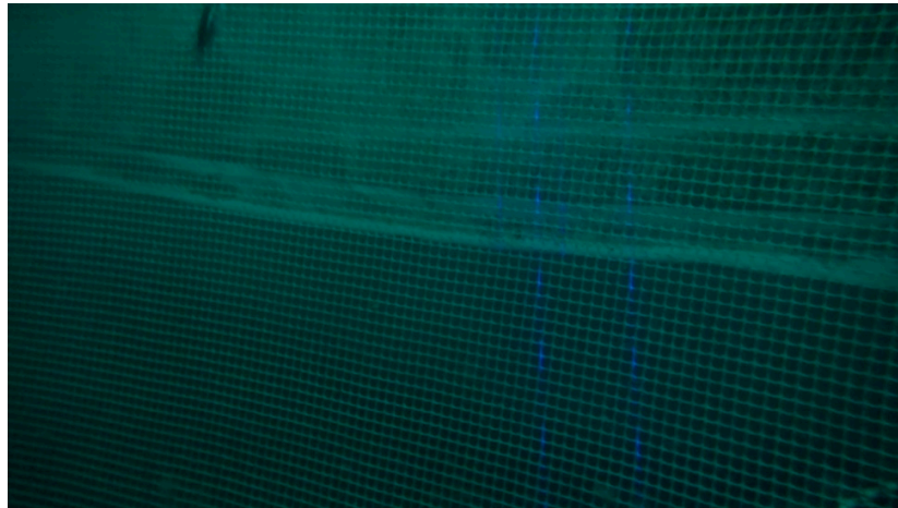
Figure 8. A picture taken at t = 650 s, where the triangulation distance disagrees with the DVL distance. The double net pen net in the upper part of the image confuses the DVL. Four laser lines are visible, two from each net.
