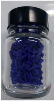
Figure 1: UTSA-16 extrudates used in this study.
