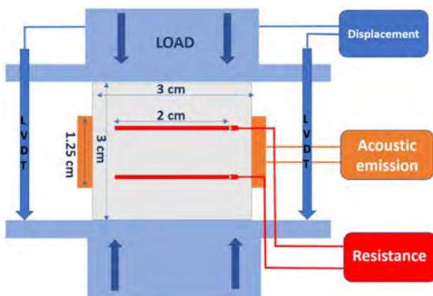
Figure 3: Schematic illustration of experimental setup (not to scale). From [19].
