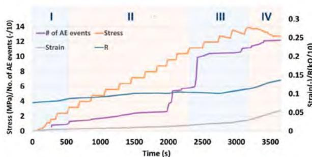
Figure 4: Resistivity changes (R) and cumulative acoustic emission events (# of AE events) upon application of mechanical load to the sample similar to that shown in Figure 1 b. The load was applied in a direction perpendicular to the surfaces of electrical connectors. Mechanical failure takes place at time of 310 seconds. From [19].
