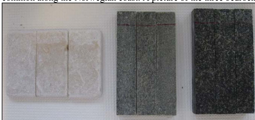
Figure 3.1-1 From left: Marble (fine structured), Shale (moderate structured), Granite (rough structured).
