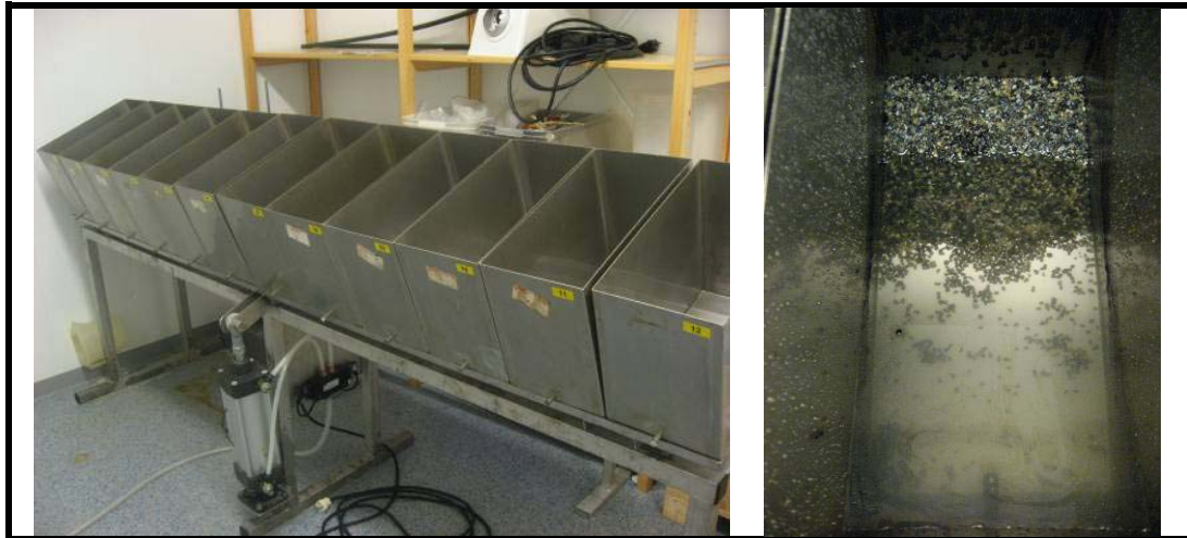
Figure 3.2-1 The shoreline simulation system (to the left) and a water reservoir with sediment (to the right).
