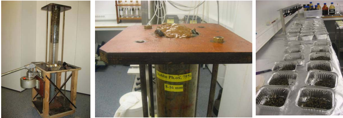
Figure 3.3-1 The hydraulic jack used for sediment sampling.
