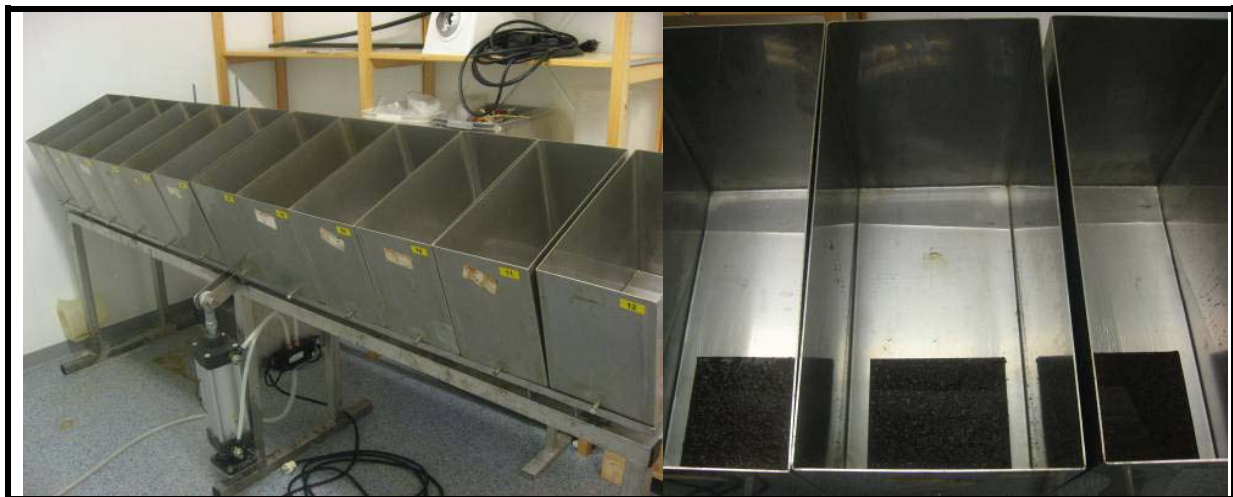
Figure 3.2-1 The shoreline simulation system (to the left) and the water reservoirs (to the right).
