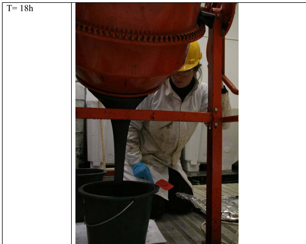
Figure 5.1 Preparation of Troll emulsions in meso-scale concrete mixer.
