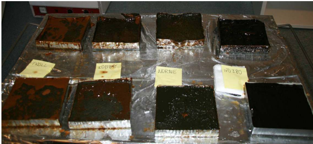
Figure 4.4: Tiles after exposure (24h) for stagnant (above) and wave action (below) for the different oil emulsions (left to right; Troll, Kobbe, Norne and IFO380) and the two different oil film thicknesses (Front row; 2mm, Back row 10mm)
