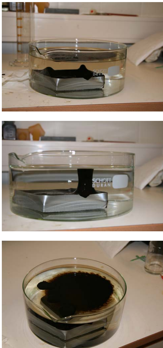
Figure 4.1: Buoyancy of bunker oil emulsion in three time steps.
