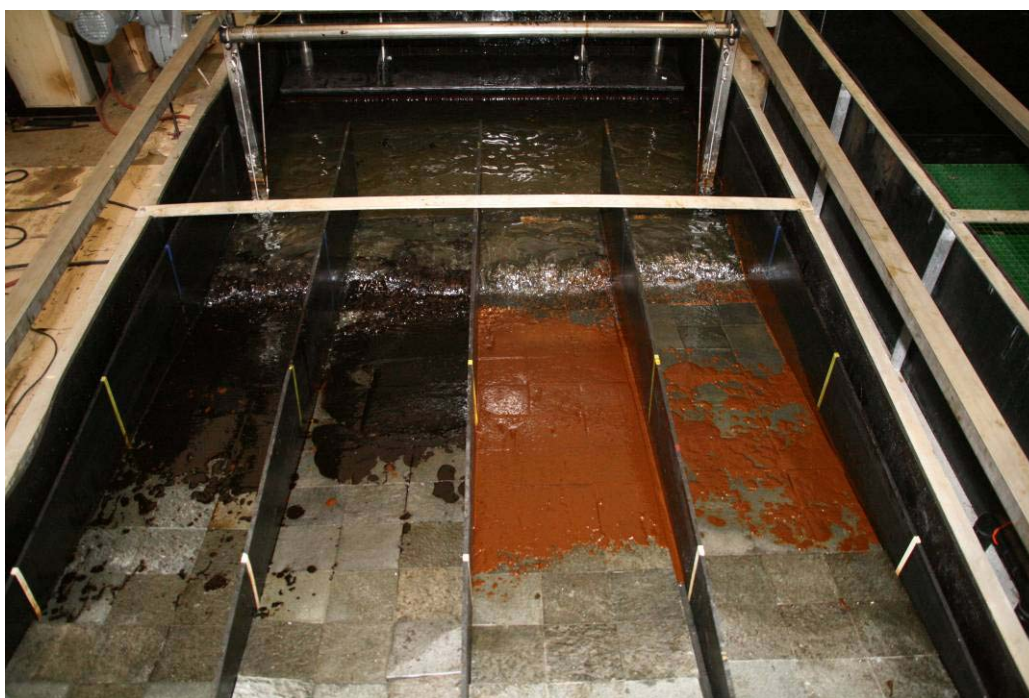
Figure 4.12; Effect of biofilm at shoreline surface on oil adhesion, 1 st low tide; from left to right; IFO380 without biofilm, IFO380 with biofilm, Troll without biofilm, Troll with biofilm
