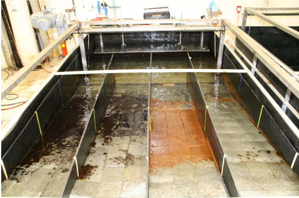
Figure 4.13; Effect of biofilm at shoreline surface on oil adhesion, 2 nd low tide; from left to right; IFO380 without biofilm, IFO380 with biofilm, Troll without biofilm, Troll with biofilm
