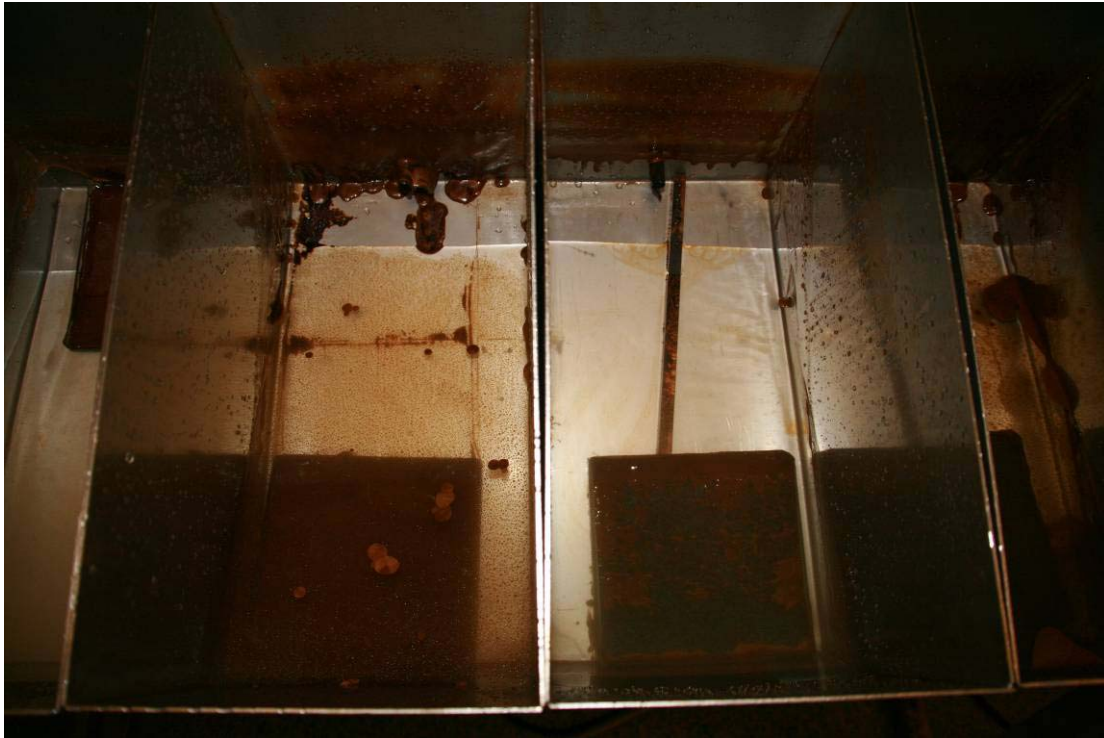
Figure 4.3: Shale tiles after exposure (24 hours) to waves action in the simulated shoreline system with mobile oil
