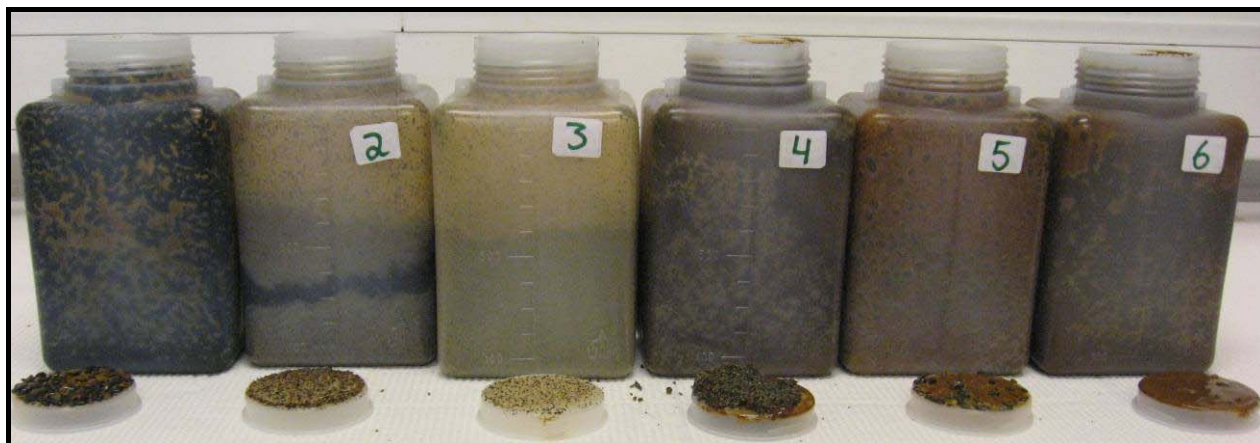
Figure 3.2-3 Sediment samples after mixing, containing different oil concentrations.
