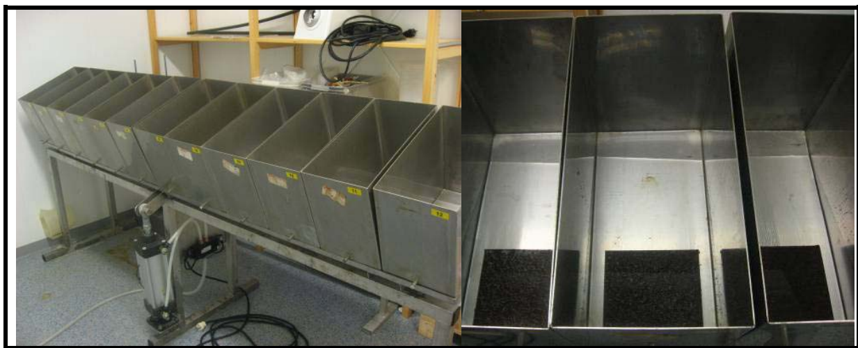
Figure 3.1 The shoreline simulation system (to the left) and the water reservoirs (to the right).
