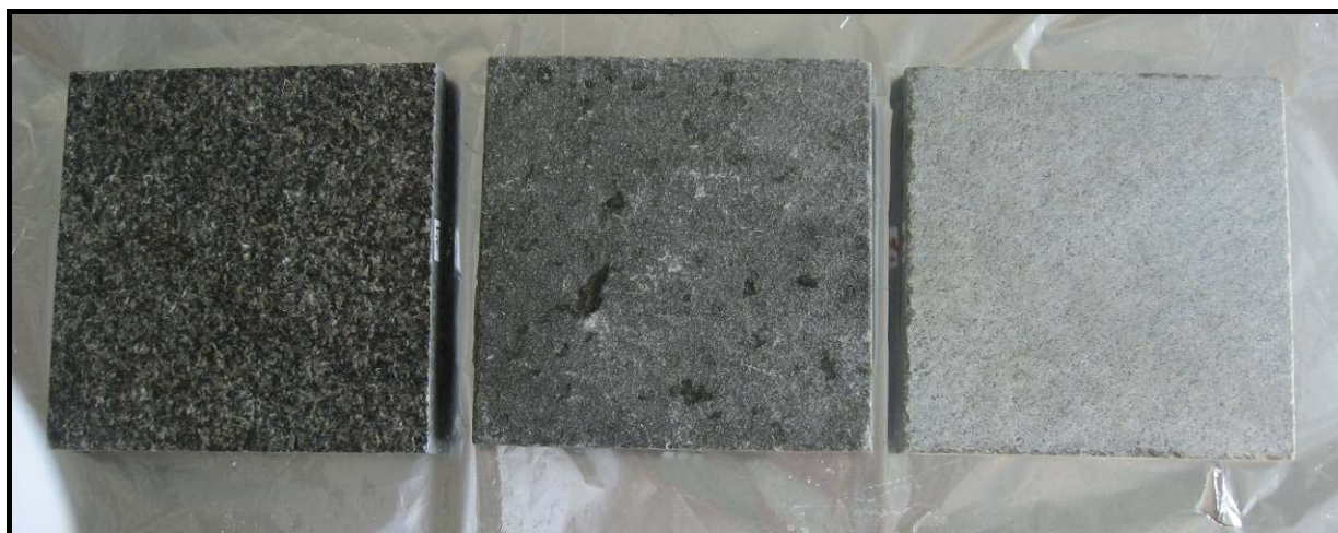
Figure 3.1-1 The tiles used in the experiments. From left: rough texture (granite), medium texture (shale) and fine texture (artificial cut shale)
