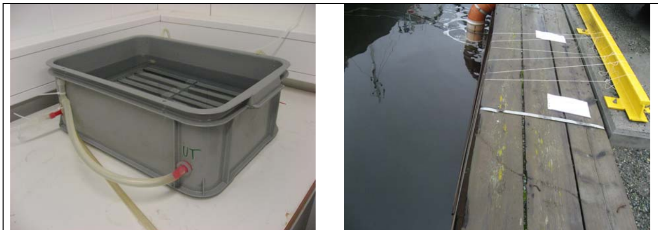
Figure 3.2-2 Method for establishment of biological film on bedrock bars, in the laboratory (left) and in the natural environment (right).
