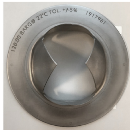
(b) After rupture.
