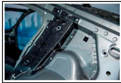
Figure 6. C-pillar from sheet molding compound (SMC, within BMW 7 series), reproduced from [157].
