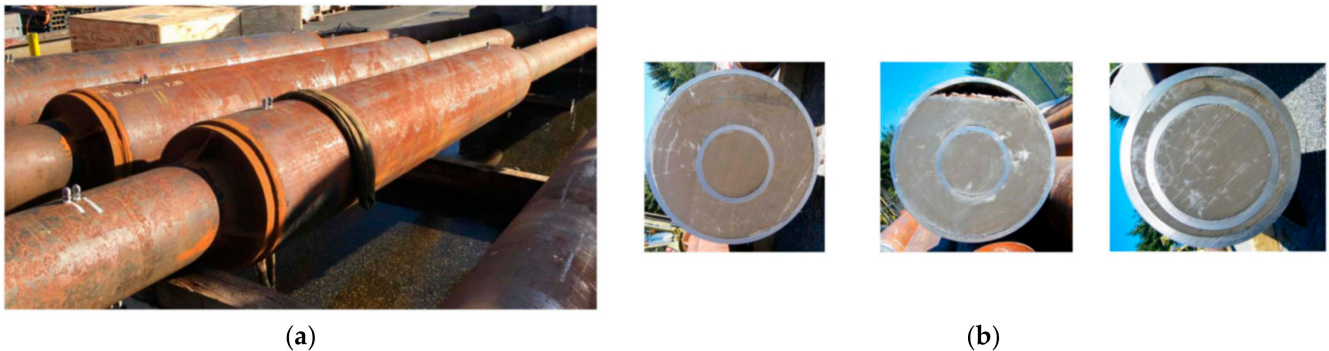
Figure 5. Cement placement test, (a) experimental setup within washout sections and (b) cut sections after cement placement from left to right: before, in, and after the washout section—Skadsem et al. [41].
