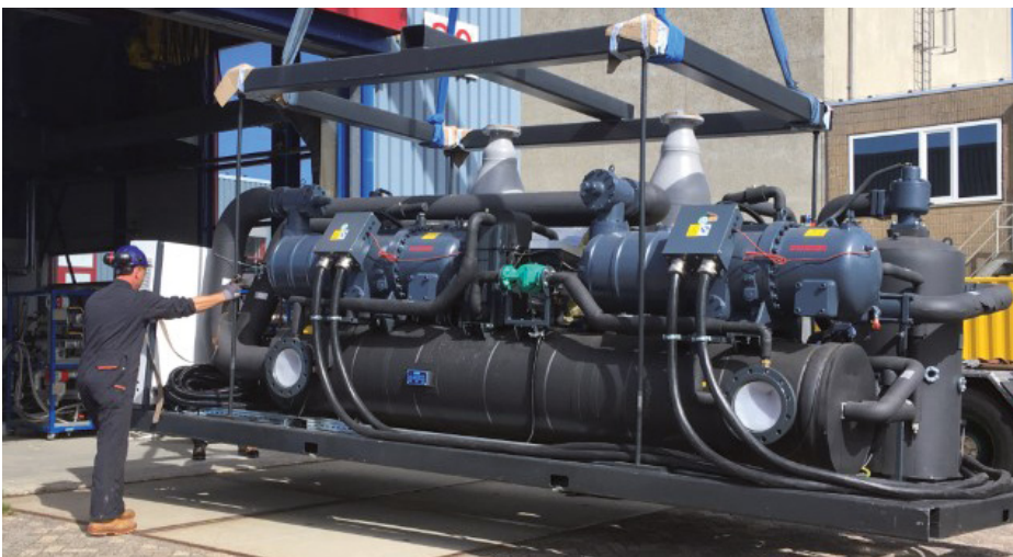
Figure 8: Heat pump developed within the framework of the LowCapex project (NL)
