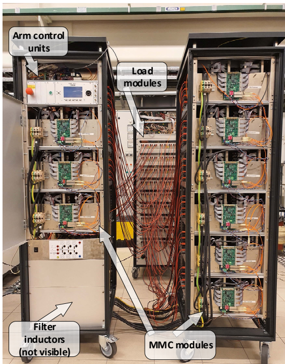
Fig. 15. Experimental setup consisting of a Modular Multilevel Converter with 12 modules per arm (the two cabinets in the front), and individual controllable loads connected to each cell capacitor (cabinet in the back).
