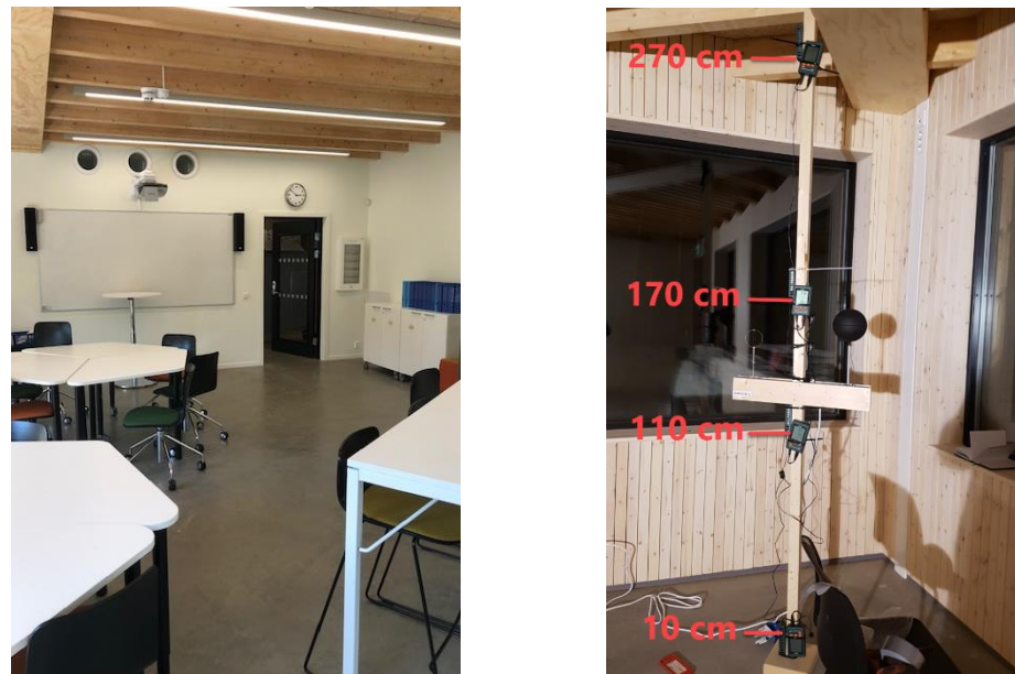
Figure 8. Photos of the classroom with measurement points for temperature and CO 2 .
