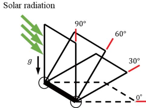
Figure 2: Schematic diagram showing how to change the tilt angle of the solar collector.
