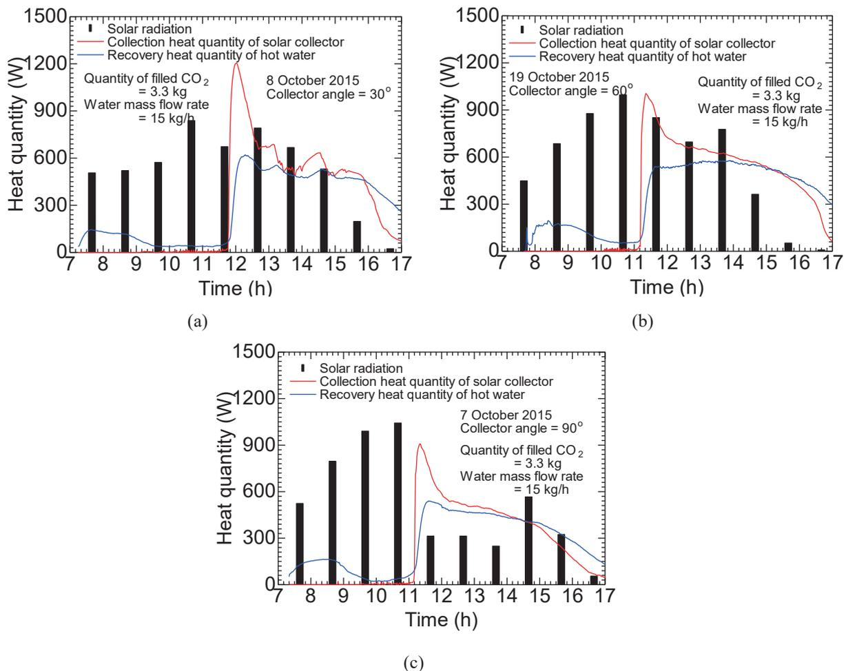
Figure 3. Solar radiation, heat quantity collected by the solar collector, and the hot water in the three representative days: (a) solar installation angle of 30° (8 October), (b) solar installation angle of 60° (19 October), and (c) solar installation angle of 90° (7 October)
