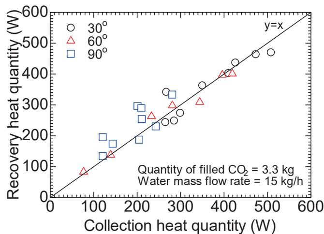
**Figure 4: Collection heat quantity of solar collector v.s. recovery heat quantity of heat exchanger with different collector angles.**
