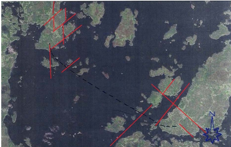
Fig. 8. Traces of weakness (red lines) in the area of tunnel crossing the Föglöfjord
