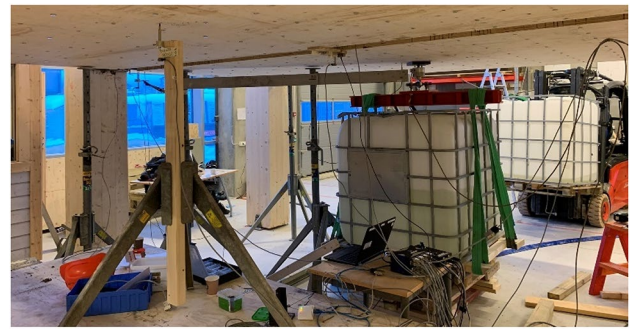
Fig. 10 Static load test situation image
