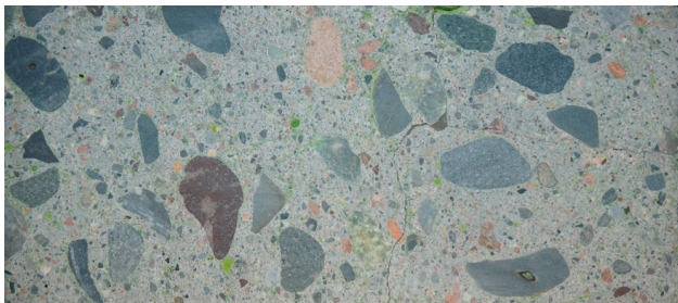
Figure 5 Plane polished section from wall section 42, in ordinary and UV-light. The length of the section is 200 mm, surface to the right. Comment: The core was drilled through a crack starting at the surface (crack width 0.25 mm), then turning parallel to the surface in a depth of about 80 mm. Due to this cracking, the outer part of the core was broken during the drilling process. The core was thus glued before preparing the polished section, with a non-fluorescence epoxy. These cracks can therefore only be observed in the left picture (but not in the right picture). [10]
