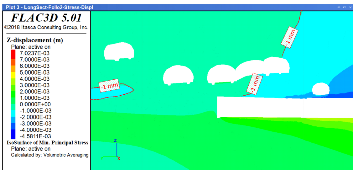
Fig. 14 Result of vertical displacement at the junction at critical excavation stage—longitudinal section along IFL tunnel
