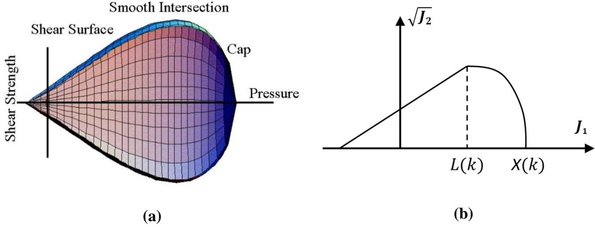
426 Fig. 8. General shape of the CSCM model yield surface in meridional plane (from Murray et
