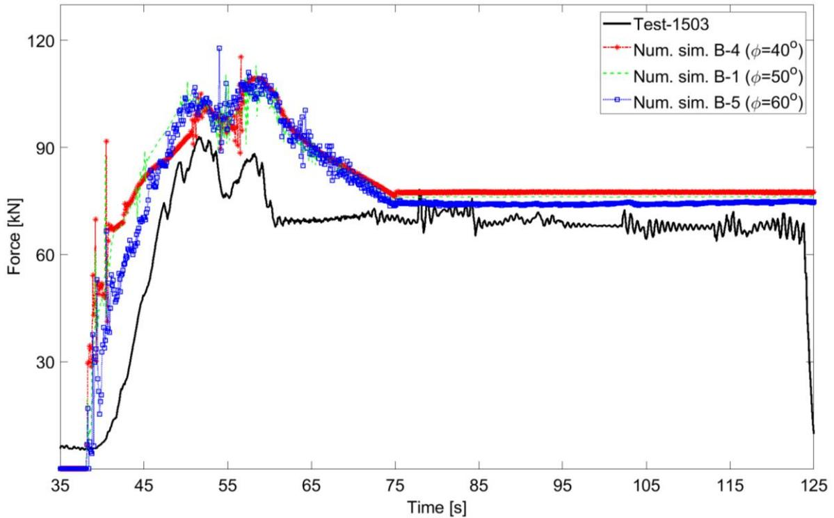
525 Fig. 11. Comparison of Friction angle ( $\phi$ ) ( $V_f=60\%$ ,  $c=0.2\text{kPa}$ )
