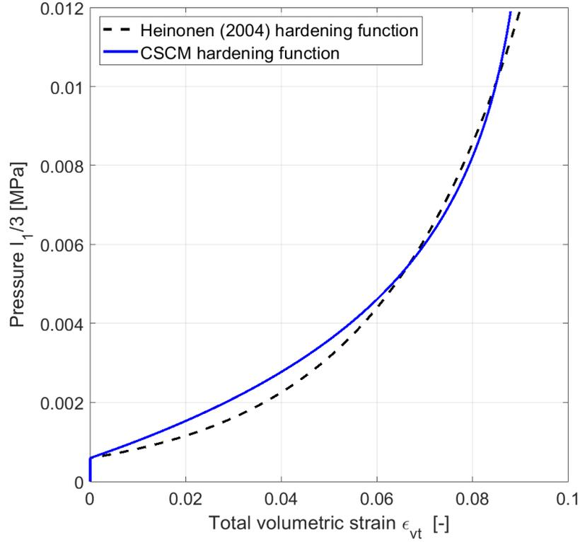
Fig. 9. Comparison of hardening function
