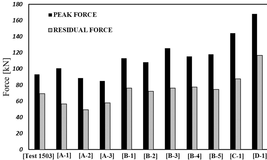
Fig. 14. The peak force and residual force for test and each simulation.
