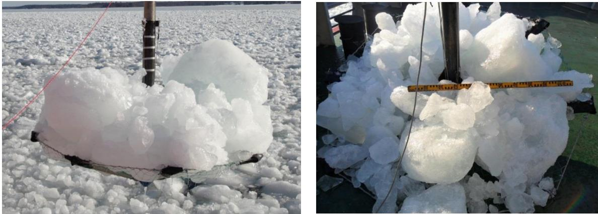
(a) Plug formed after collector is completely removed from the water and is hanging in the air
