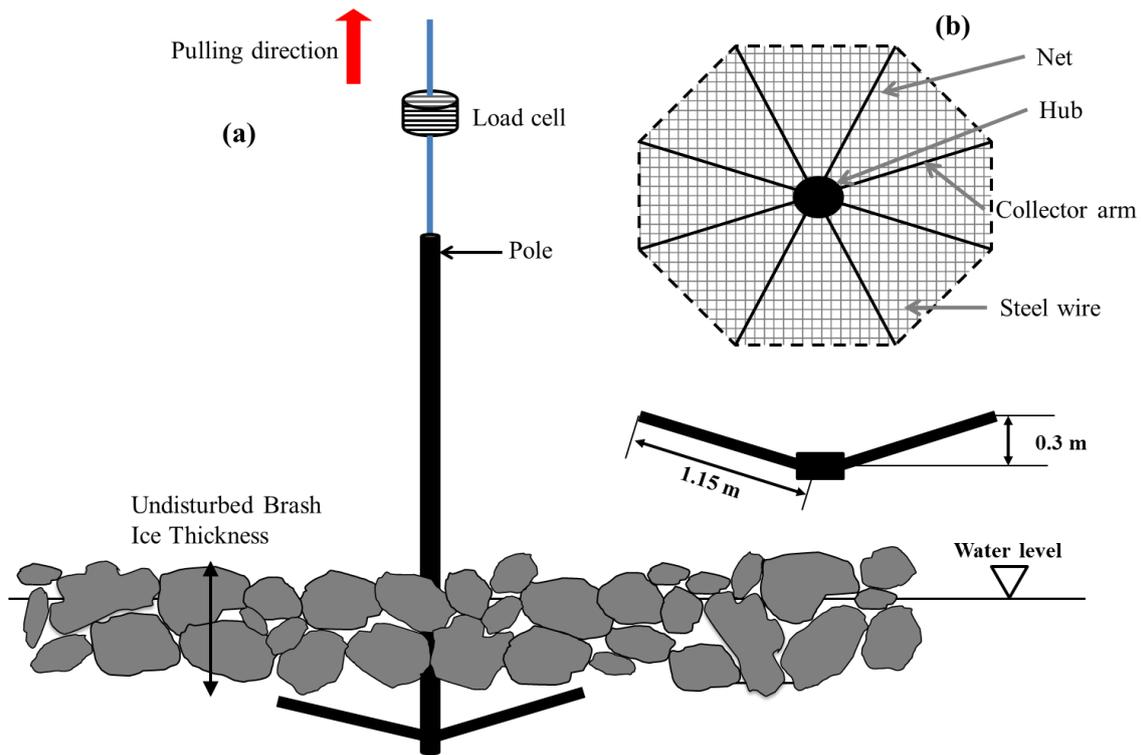
Fig. 2. (a) Schematic of the pull-up test (b) Parts of the collector.
