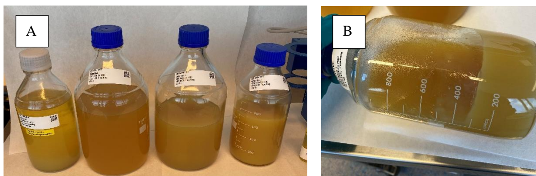
Figure 3-3 A: From left to right: fresh oil, 150°C+, 200°C+ and 250°C+ residues. B: 250°C+ residue with visible wax precipitation
