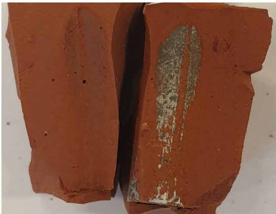
Figure 10 – Split sample of aluminium reinforced binder with 50% AR-BR.
