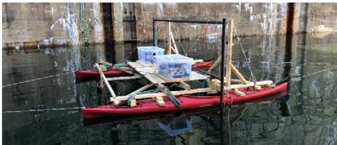
FIGURE 1: TEST RIG. RAFT CONSISTING OF TWO KAYAKS AND A TIMBER FRAME. FRAME RESTING ON BRACKETS (PIVOT POINTS). PICTURE SHOWING RAFT AT REST. TOWING DIRECTION TOWARDS THE LEFT.
