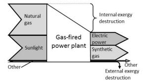
**Figure 3:** Grassmann diagram for the gas-fired power plant with CO<sub>2</sub> chemical absorption and bio-gas conversion.
