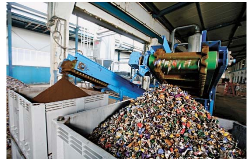
Figure 19: facility for recycling of coffee capsules
