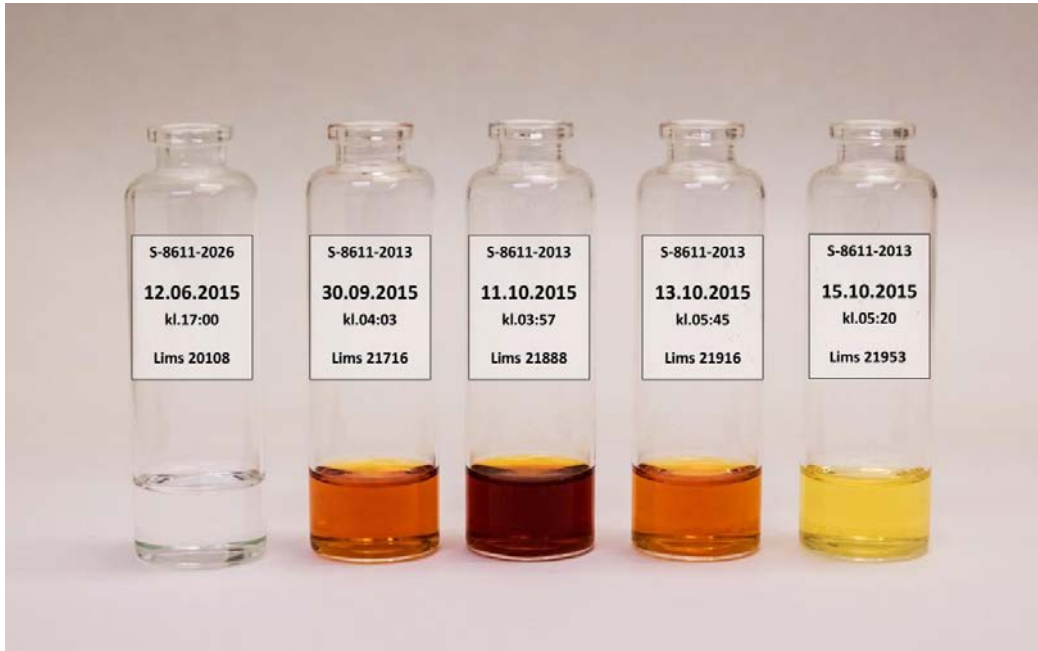
Figure 4: Picture of solvent samples taken during the campaign. The color change indicates solvent degradation.
