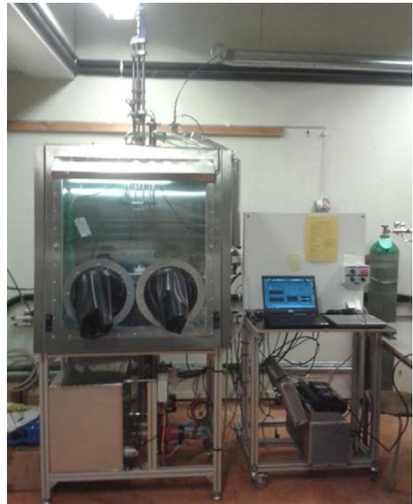
Figure 2: Thermally insulated glove box with oxide skin strength measurement apparatus. The cooling water temperature is adjusted to be able to increase water vapor in the atmosphere.
