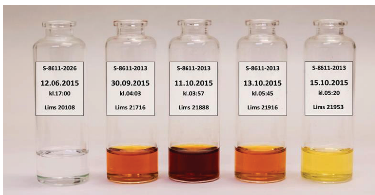
Figure 4. Pictures of samples taken during the campaign. The color change gives an indication on how degraded the solvent is. The samples are from left to right after: 0, 1300, 1830, 1870 and 1920 hours of operation.
