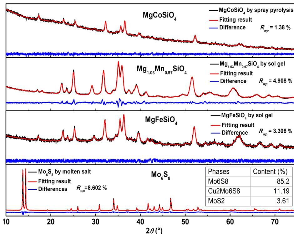
Figure S1. Typical Pawley fitting of the XRD patterns for MgMSiO<sub>4</sub> (M=Fe, Mn, Co) and Rietveld refinement for chevre phase Mo<sub>6</sub>S<sub>8</sub>.
