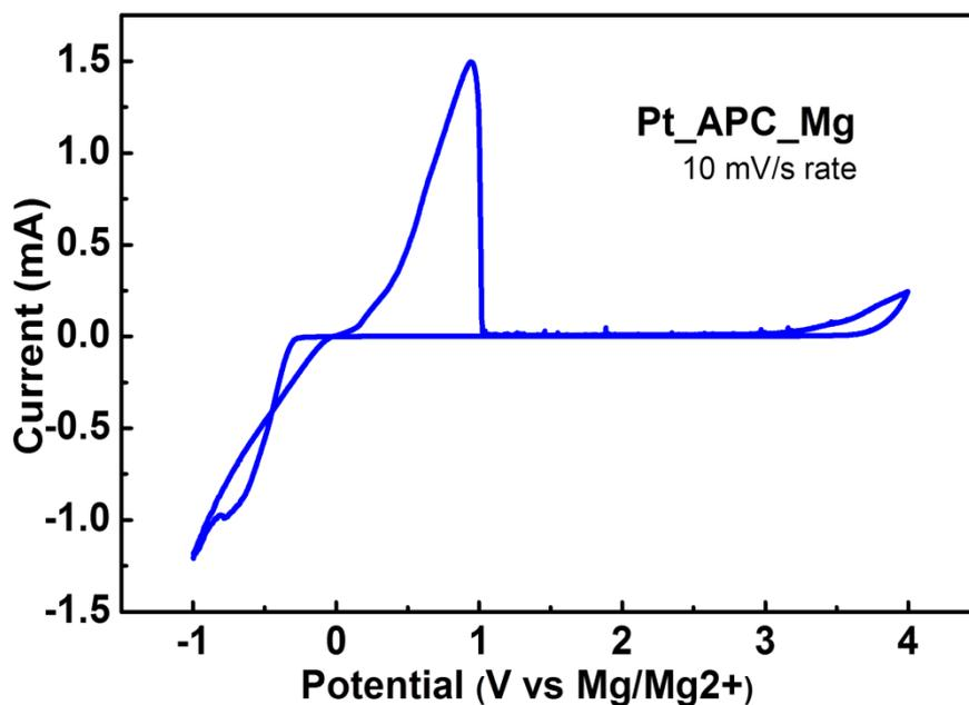
Figure S2. Cyclic voltammogram of APC solution by using Pt as working electrode and Mg strip as counter/reference electrode at a scan rate of 10 mV/s.
