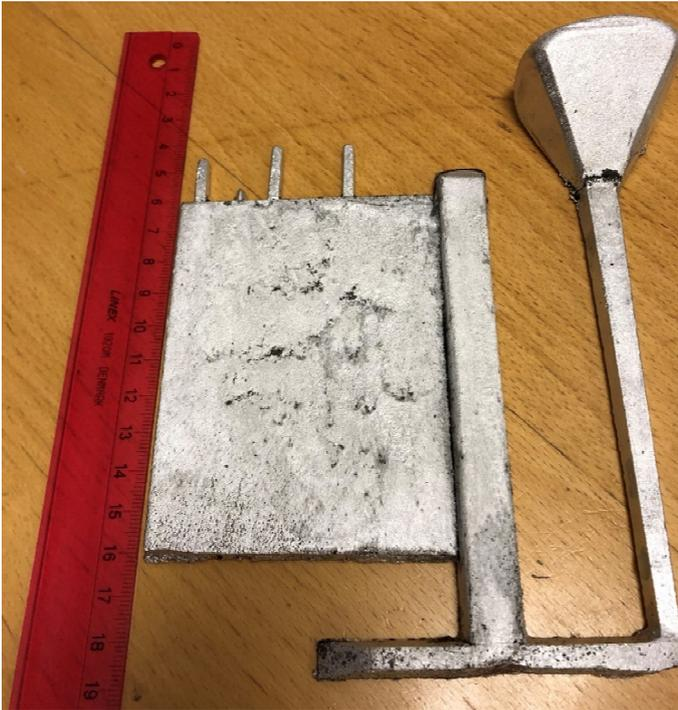
**Figure 3 Samples in as cast form.**
