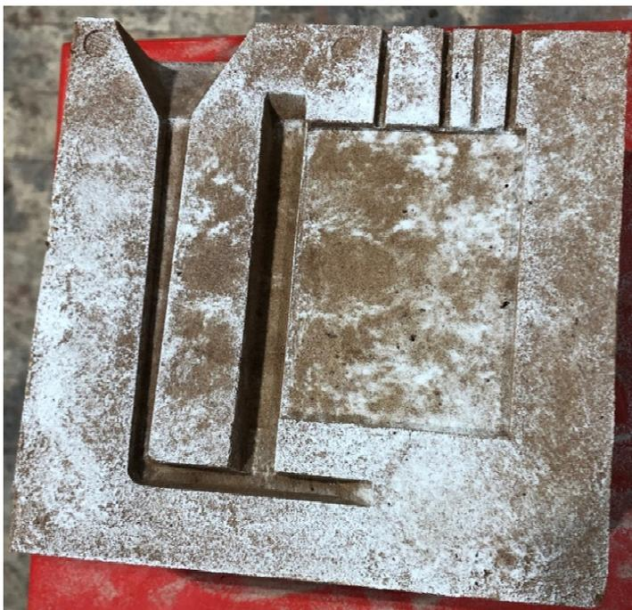
Figure 2 Sand mold used for casting samples.
