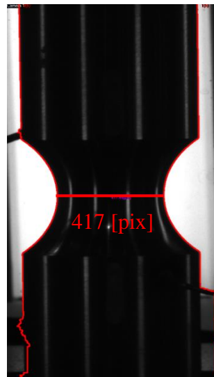
Fig. 6 Specimen image edges in Fig. 5 (a) derived with the edge tracing method. The minimum cross-section diameter is also shown in pixels.
