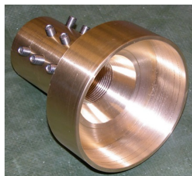
Figure 1. End cap used to seal off the ends of the 5-m long MIND cable samples used in the present study. It was machined out of a \varnothing=150 mm brass cylinder.
