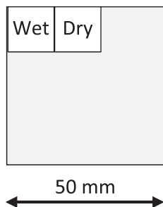
Fig. 2. The basic samples (large square) were ca. 50 × 50 mm 2 and cut from the upper part of the crucibles. The specimens subjected for bubble analysis were ca. 12 × 12 mm 2 and cut from the basic samples as shown above.
