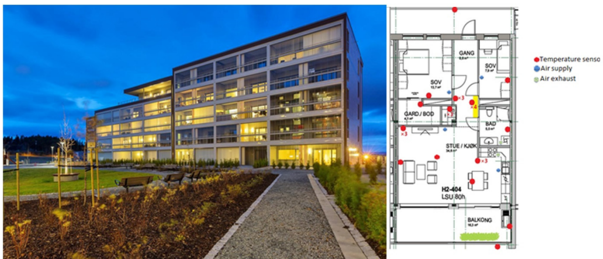
Figure 23 Typical configuration investigated with one-zone ventilation and a radiator (in yellow) placed in a central position. Picture of the apartment block investigated in Miljøbyen Granåsen (image: Interiørfoto [62]).
