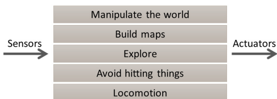
Figure 6. Layered control system according to Brooks [19]
