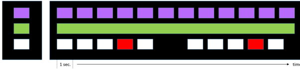
Figure 6. Example of automation transparency: Left, the three self-driving mode signals. One over the other. Right, a time diagram of the flash sequences described in detail in the text.
