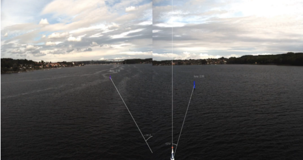
Fig. 9. Object detection and classification on two RGB images are shown by highlighting the detected object in green colour and showing the bearing to detected objects.
