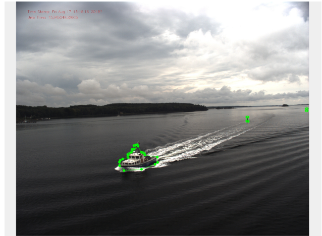
Fig. 5. Green polygons show the boundaries for one boat and two buoys that are present in this image.
