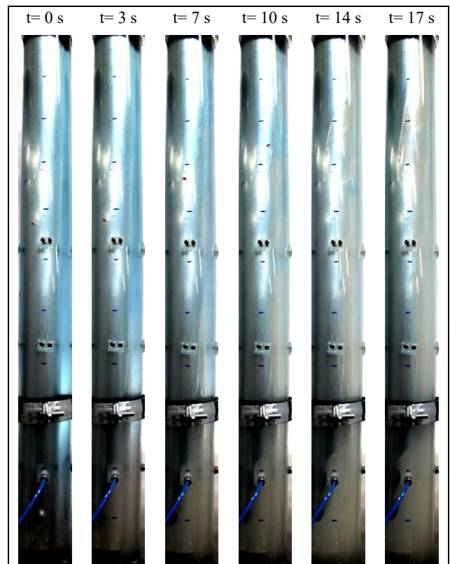
Figure 8: Snapshots of Displacement Flow in Test no. 12
