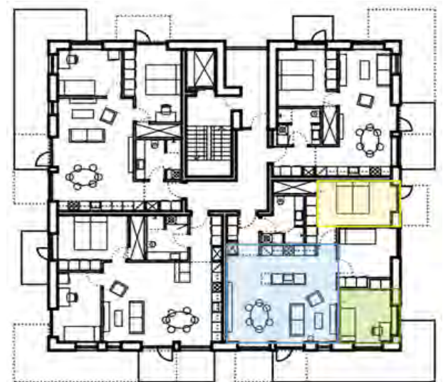
Figure 2 Floor plan with indication of rooms selected for thermal comfort evaluation (green, blue) and daylight availability (blue, yellow). Illustration: TRANSFORM.
