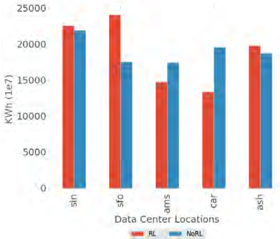
Figure 4: Total Site annual energy for statically (NoRL) configured IT load and dynamically reset (RL) IT loads.
