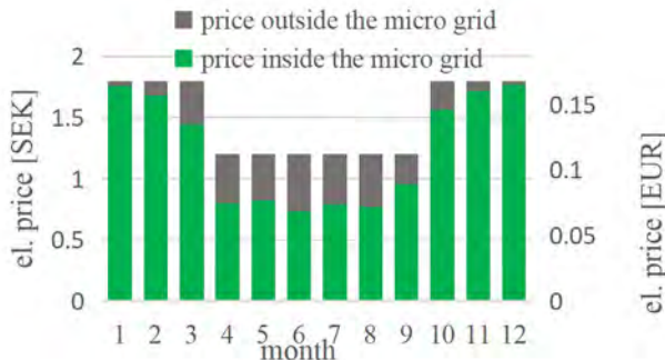
Figure 5: monthly difference in price between the energy offered by the parent grid and the average paid by the shareholders in a LEC gratis arrangement.
