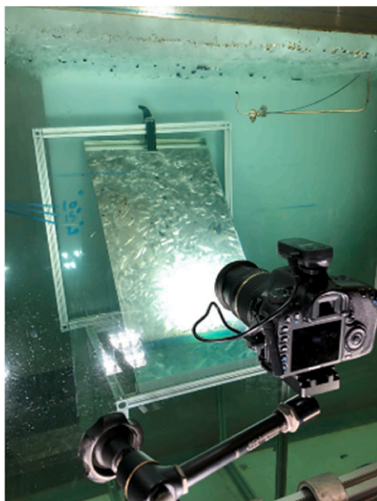
Fig. 3. Picture of the SLR camera mounted outside the flume window taking pictures from underside the ice through a 45° mirror.
