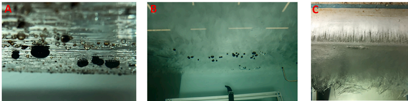
Fig. 4. Pictures of the ice structures used in testing of horizontal movement of oil droplets under ice. A: Smooth ice; B: frazil ice; C: skeletal ice layer.
