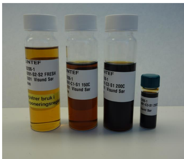
Figure 3-4 Visund Sør from left to right: Fresh oil and residues (150, 200 and 250°C+)
