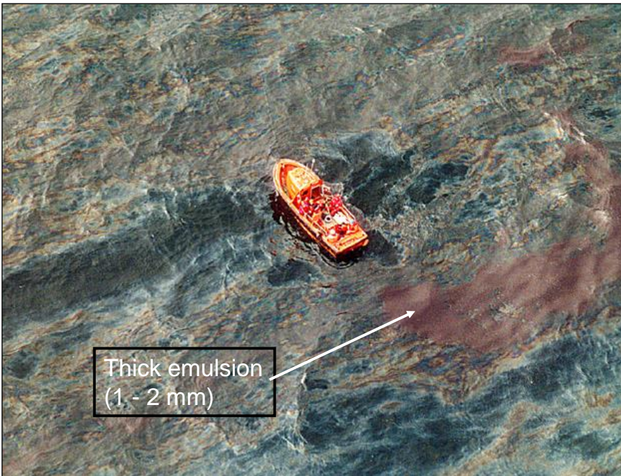
Figure A-6 Surface oil slick (initial thickness > 200 \mu\text{m} ) from the experimental deep-water release "DeepSpill" in 2000. Surface oil is emulsifying like an oil slick from a surface batch release (from Leirvik et al., 2011)
