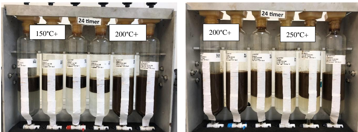
Figure 3-7 Rotating cylinders of water-in-oil (w/o) emulsions of Visund crude oil after 24 hours at 13 °C
